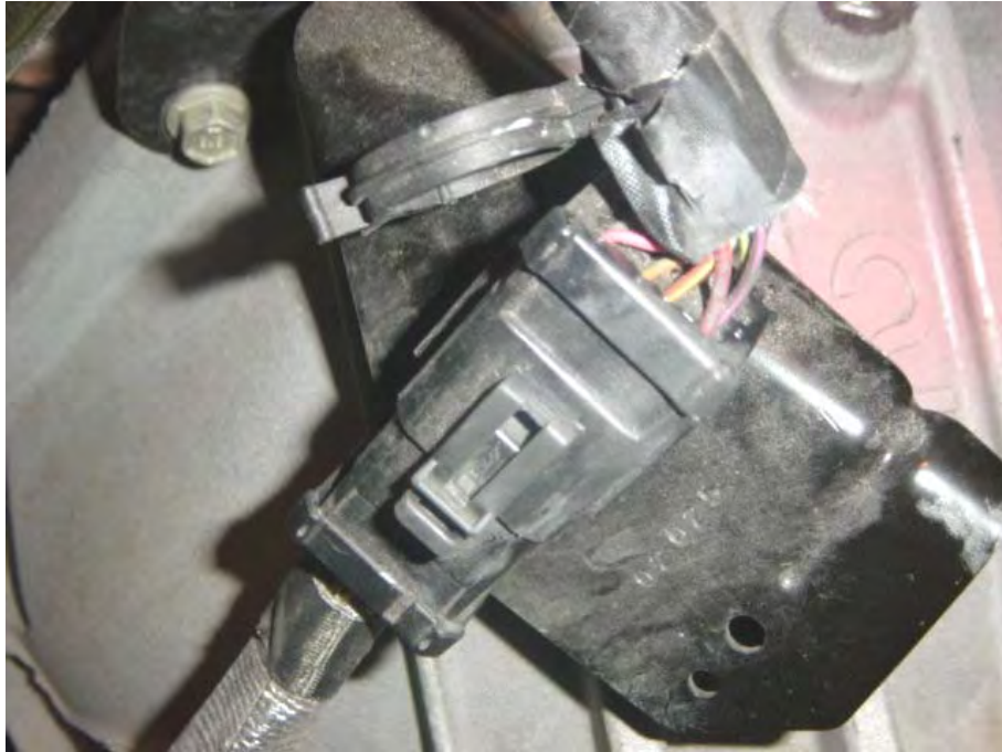
CHAFFED WIRE IN TRANSMISSION HARNESS (1,889 TEST MILES)
