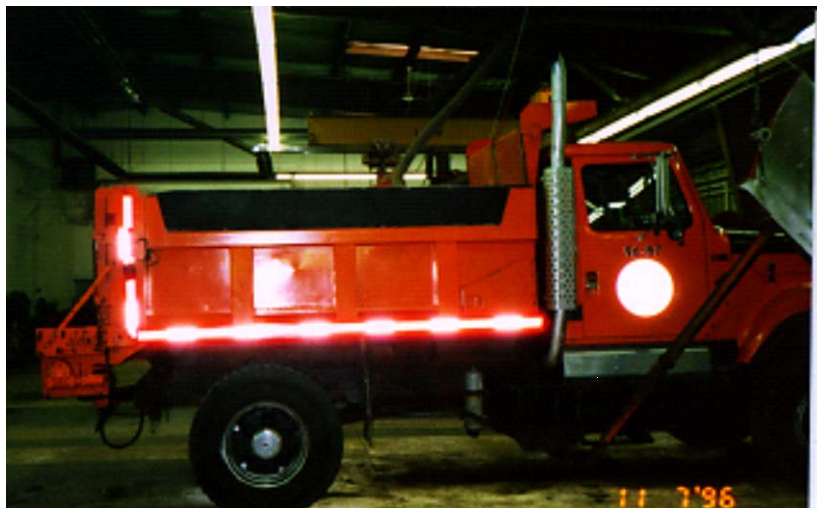
Figure 1. A small patrol truck showing the inverted “L” shape.
