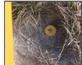
Figure 24. RAW monument with yellow cap and yellow plastic post with sign nearby. Posts may be metal too.
