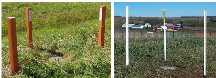
Figure 45. Orange guard or white witness posts surround a typical geodetic survey control monument station installation. Some of these monuments may have only 1 or 2 posts.
