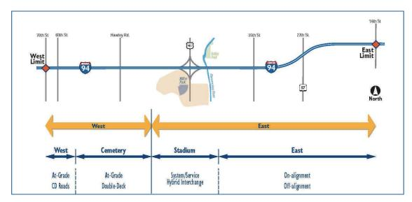
All of these build alternatives are interchangeable. For example, both the On-alignment and Offalignment alternatives in the east segment are compatible with the Double Deck alternative in the west segment. The same holds true for the At-grade alternative. The four alternatives are:
