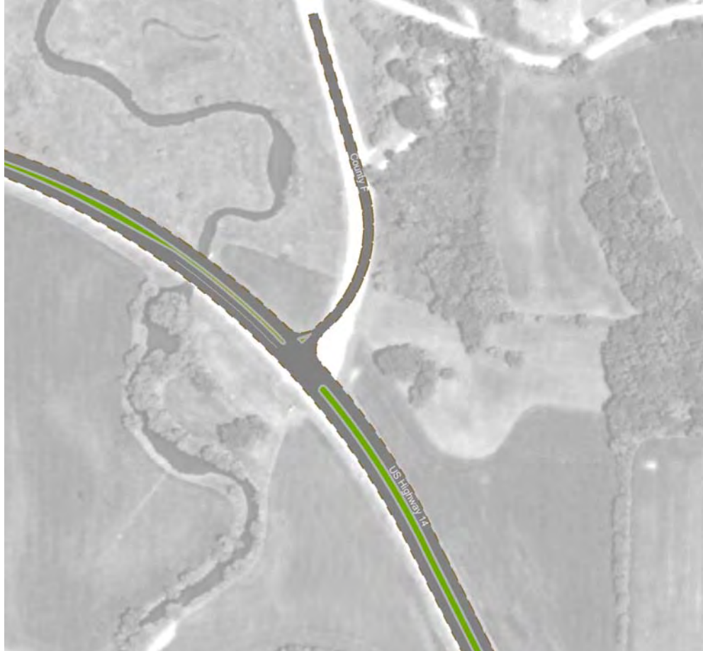
Figure 18 Proposed intersection improvements at County F
