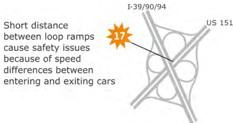
Figure 19. Short Distance Between Loops Ramps US 151
