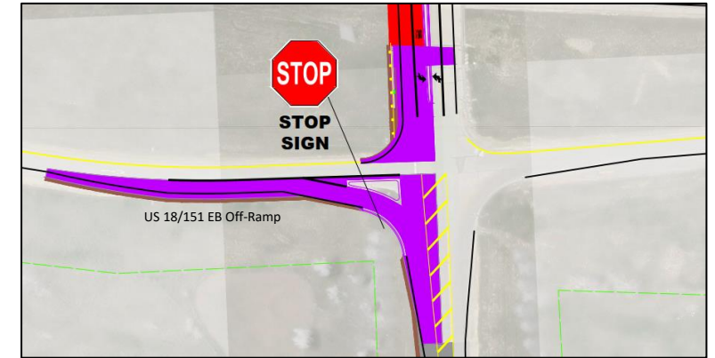
Side-road Stop Control Alternative
