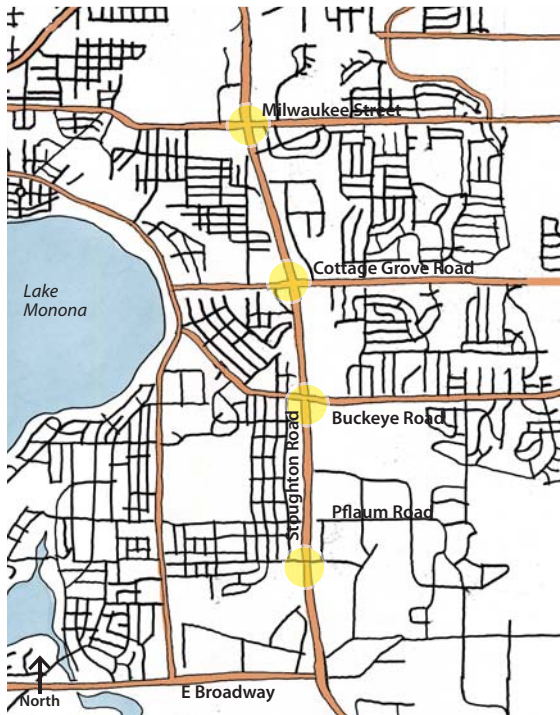
Intersections: Intersections along Stoughton Road (yellow) and the cross streets process three types of high volume traffic. Additional street networks that serve local trips would reduce congestion and intersection delay by providing alternative routes.
