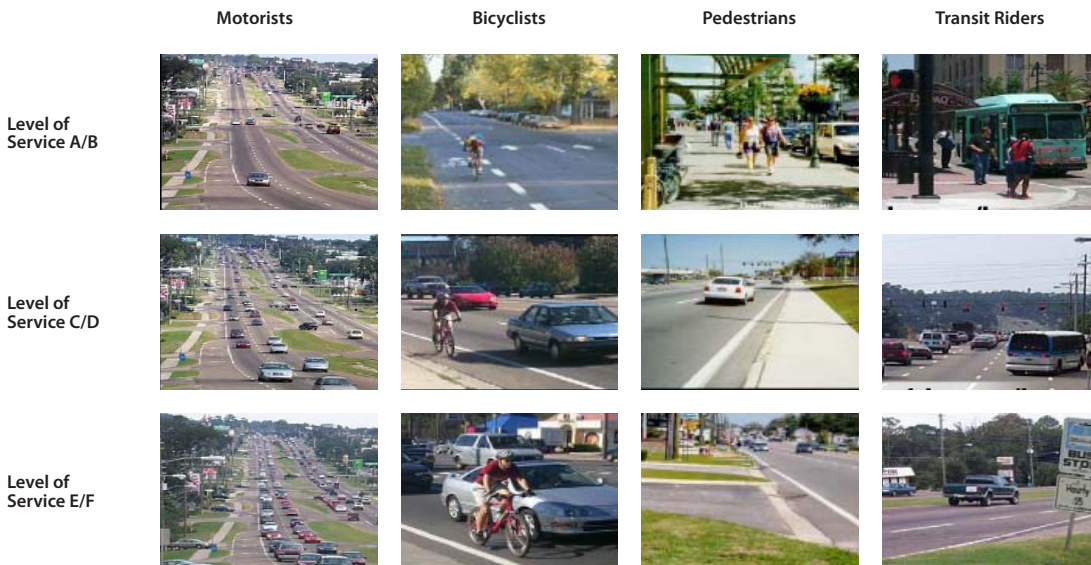
Level of Service: Level of service for streets and intersections should apply to multiple users.
