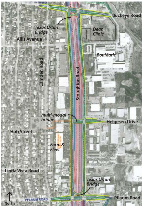
WisDOT Alternative B: Stoughton Road is depressed between Buckeye Road and Pflaum Road.
