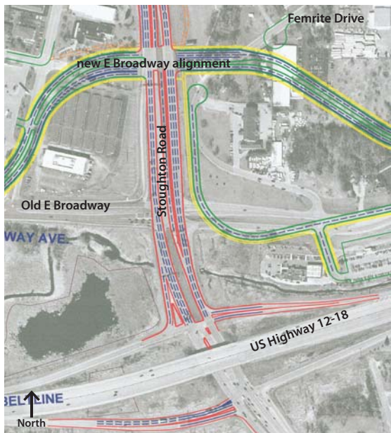
Non-Flyover Alternative: WisDOT Alternative A maintains an at-grade condition at East Broadway and Stoughton Road, and adds a third left turn lane to the eastbound exit ramp from U.S. Highway 12-18 to northbound Stoughton Road.
