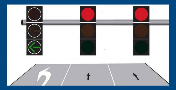
Signalized intersections with a high frequency of angle crashes that involve left turning and oncoming vehicles are expected to have fewer crashes with protected left turn signal phasing since opposing traffic is restricted from entering the intersection.
