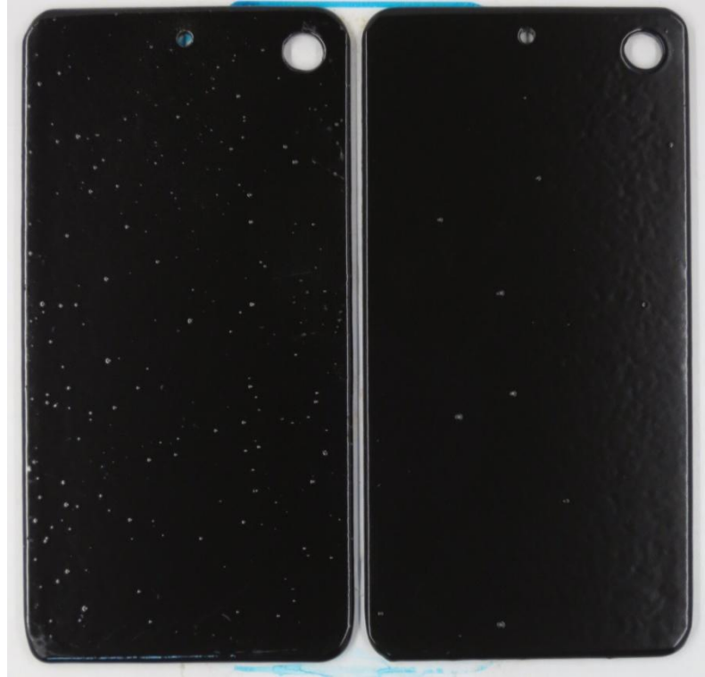
Figure 48: Initial (left) and Final (Right) Out-gassing Craters
