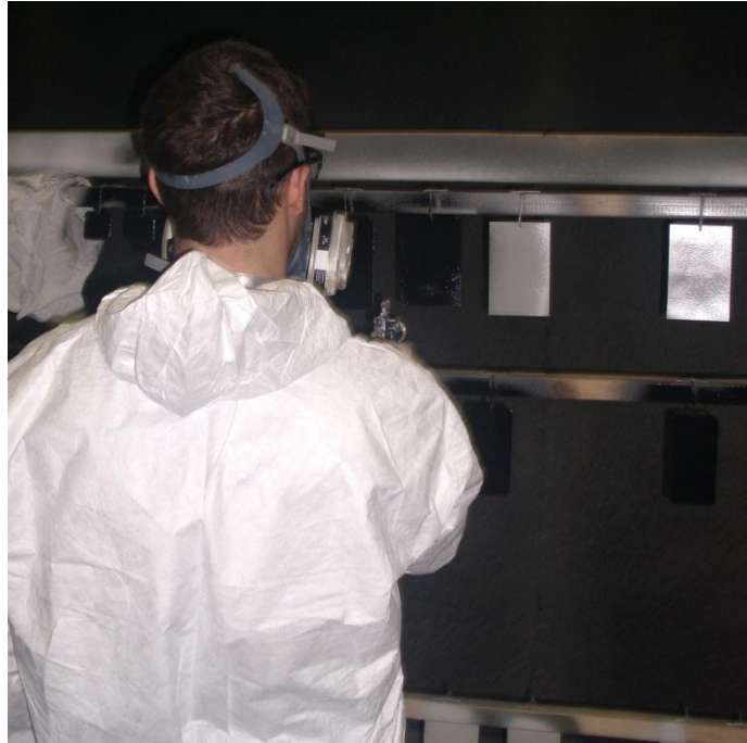
Figure 47: Application of Top-Coat
