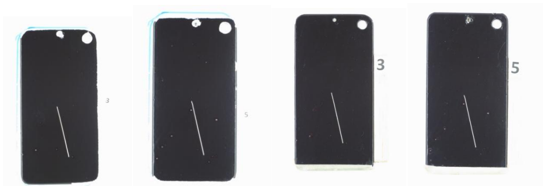
Figure 86: SW-05PD Initial and Final Creepage
