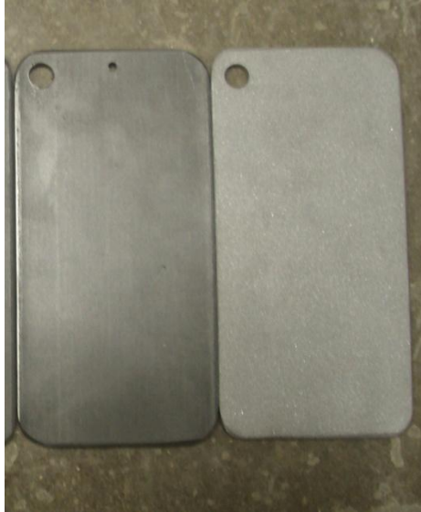
Figure 39: Surface Preparation Prior to Galvanizing
