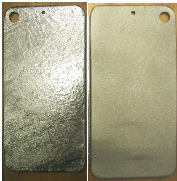
Figure 40: Galvanized Brush-Off Blasting.
