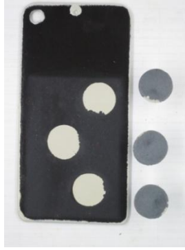
Figure 96: Final Adhesion Failure SW-PD04
