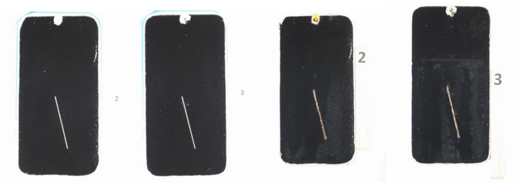
Figure 85: SW-3F Initial and Final Creepage
