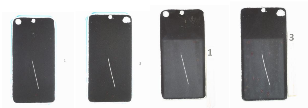
Figure 87: SW-04PD Initial and Final Creepage
