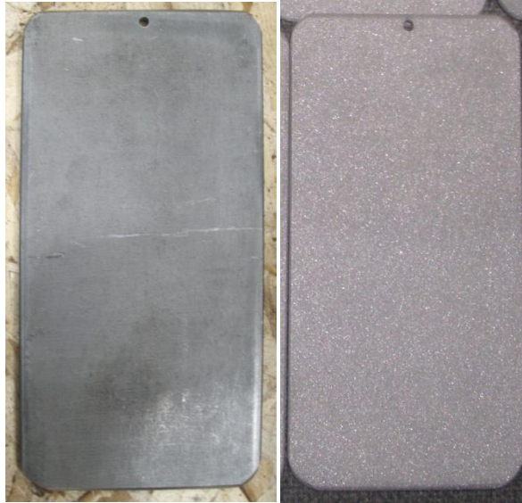
Figure 36: Sample Before and After Sandblasting
