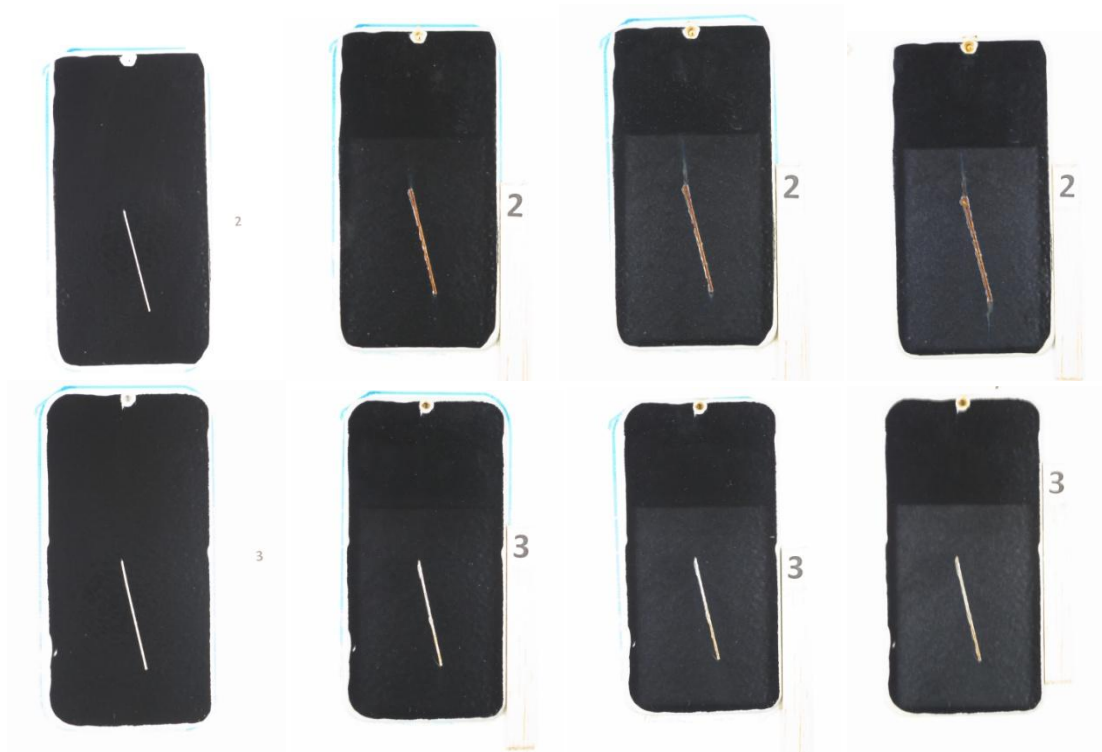
Figure 80: SW-3P Initial, Cycle 9, Cycle 12, Cycle 15
