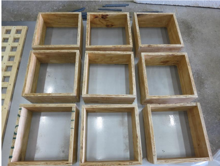
Figure 0-1: Typical concrete sample formwork.
