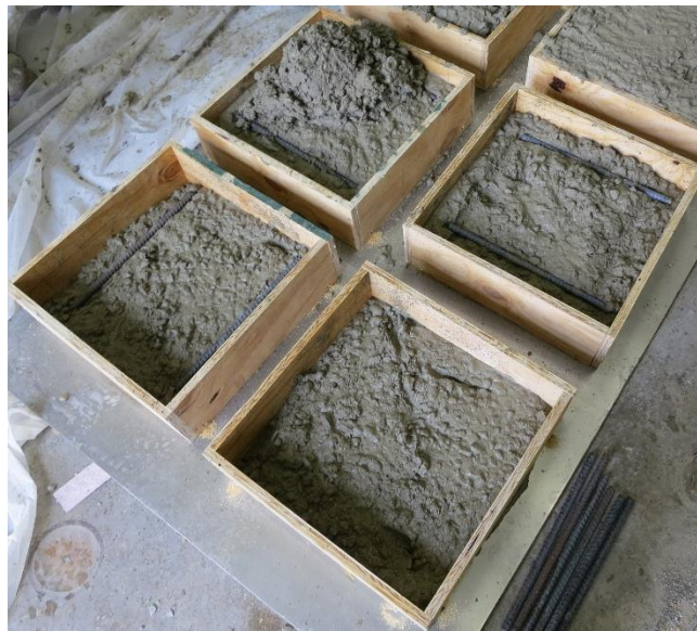
Figure 0-2: Typical reinforcement of the chloride ion and outdoor exposure test specimens.
