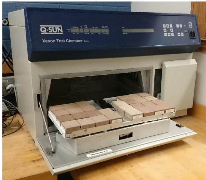
Figure 0-13: Xenon Arc test chamber, with an uninsulated black panel for temperature measurement.
