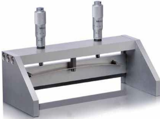
Figure 0-22: Adjustable film casting knife (Left) and a prepared permeability dish with test specimen (Right).
