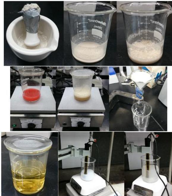
Figure 0-20: AASHTO T-260 evaluation procedure.
