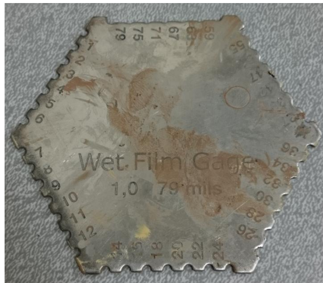
Figure 0-5: Wet film gage used during coating application.
