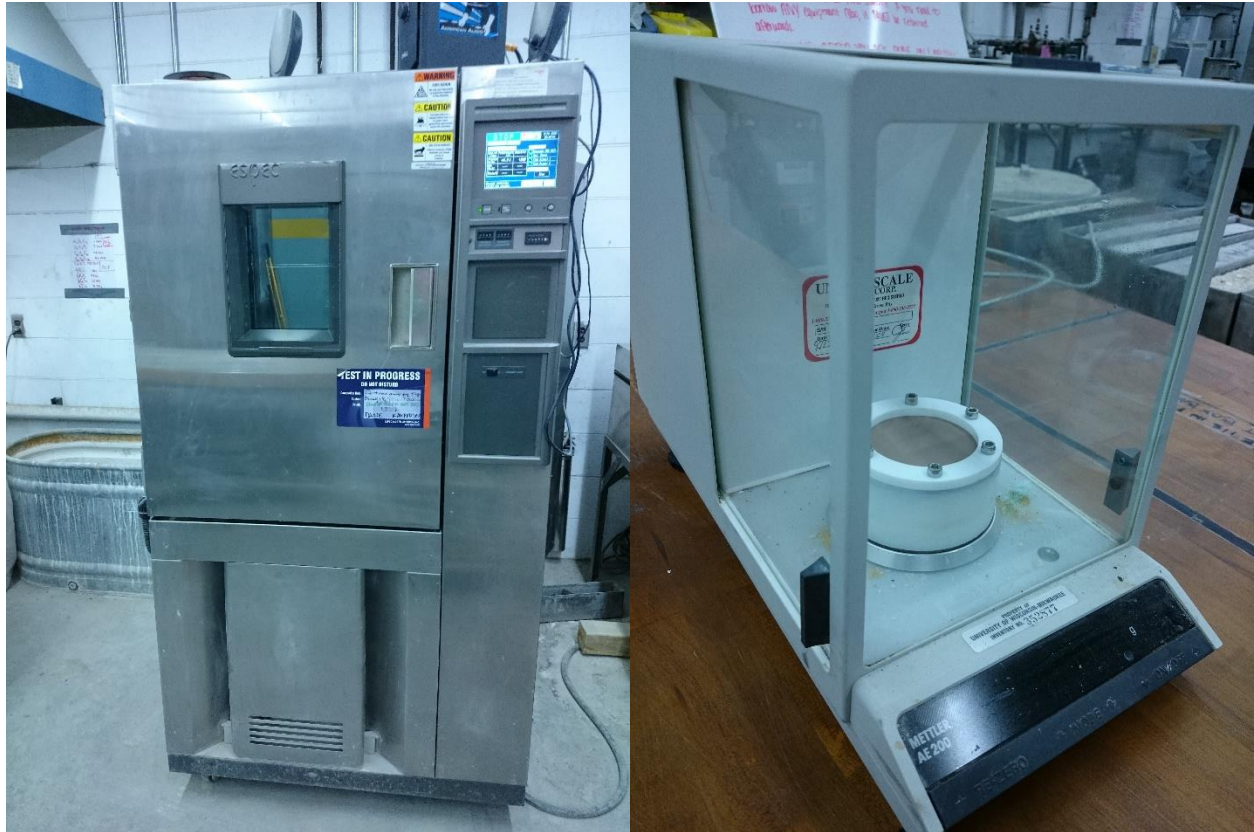
Figure 0-23: Environmental chamber (Right) and scale (Left) used for the evaluations of water vapor transmission.
