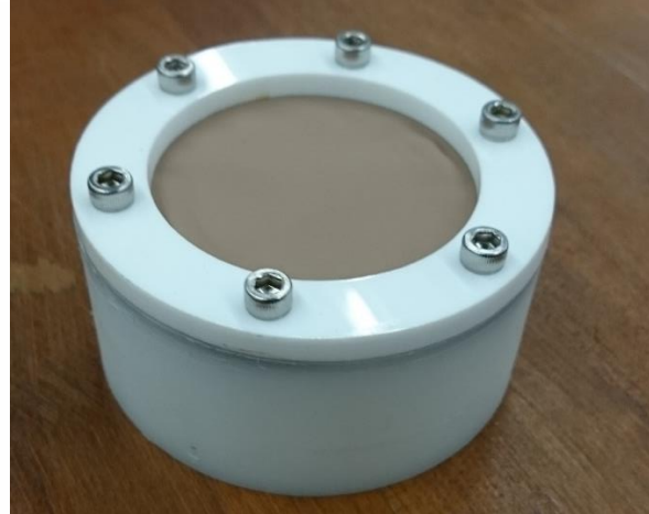
Figure 0-22: Adjustable film casting knife (Left) and a prepared permeability dish with test specimen (Right).
