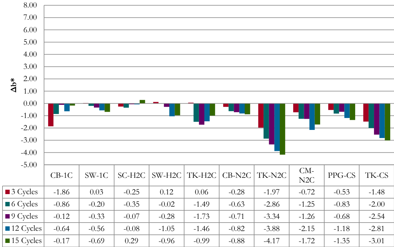
Figure 0-12: Mean values of \Delta b^* of each coating system throughout xenon arc exposure.
