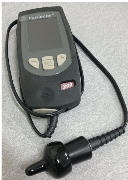
Figure 0-16: Ultrasonic coating thickness gage used to determine dry film thickness.
