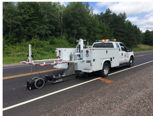
Evaluating the structural capacity of HMA pavement using a Falling Weight Deflectometer
