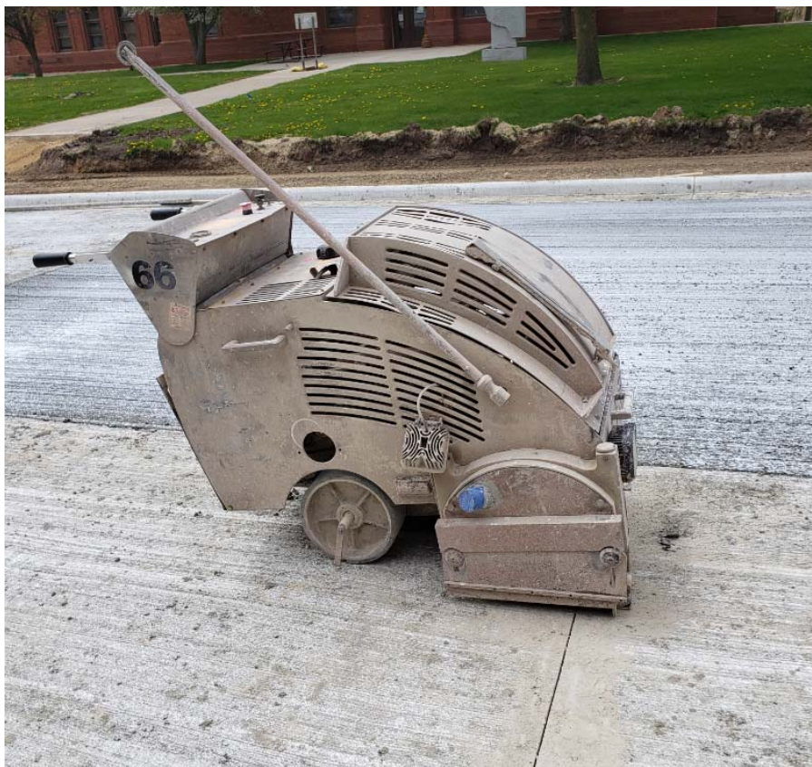
Figure 2.3.5: Husqvarna 4200 Soff Cut Early Entry Green Saw
