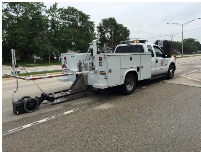
FWD testing on WIS 100 with RCA base layer
