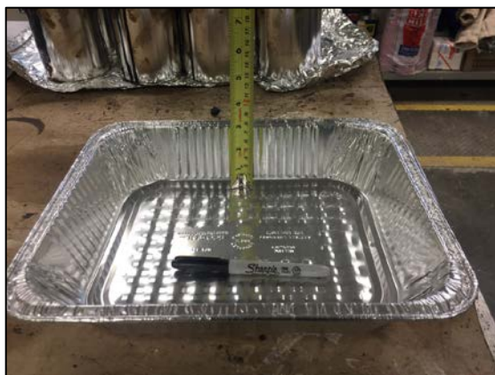
Figure 14. Typical Pan Used to Preheat/Age Loose Mixture for This Study.
