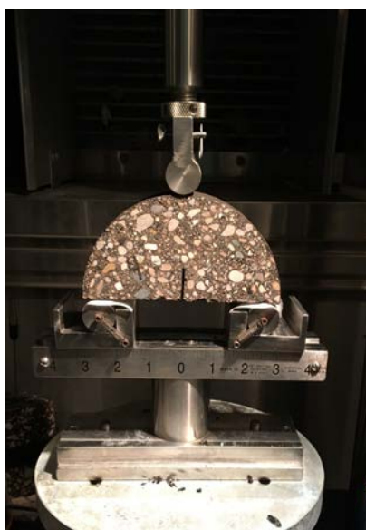
Figure 15. General Test Setup of an SCB Sample.
