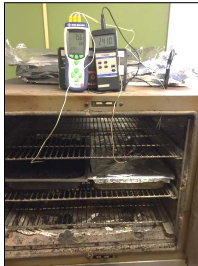
Figure 4. Monitoring Temperature of Covered versus Uncovered Samples.
