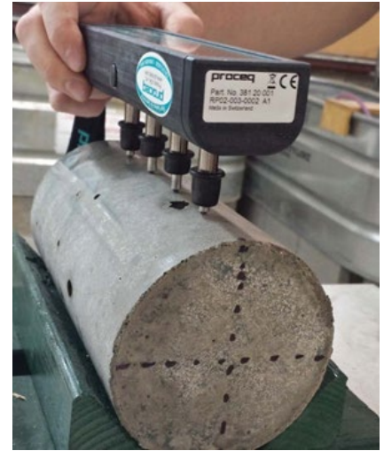
Conducting a surface resistivity test
