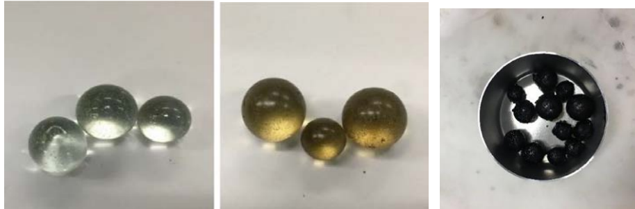
Figure 6 Glass Beads; (a) Before Mixing, (b) After Dry Blending with RAP only, (c) After Normal Mixing with Virgin Binder, Virgin Aggregate, and RAP
