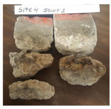
Figure 15. Cores from buckling sites taken from transverse joints and core holes showing spalls in the lower portion of the joint.
