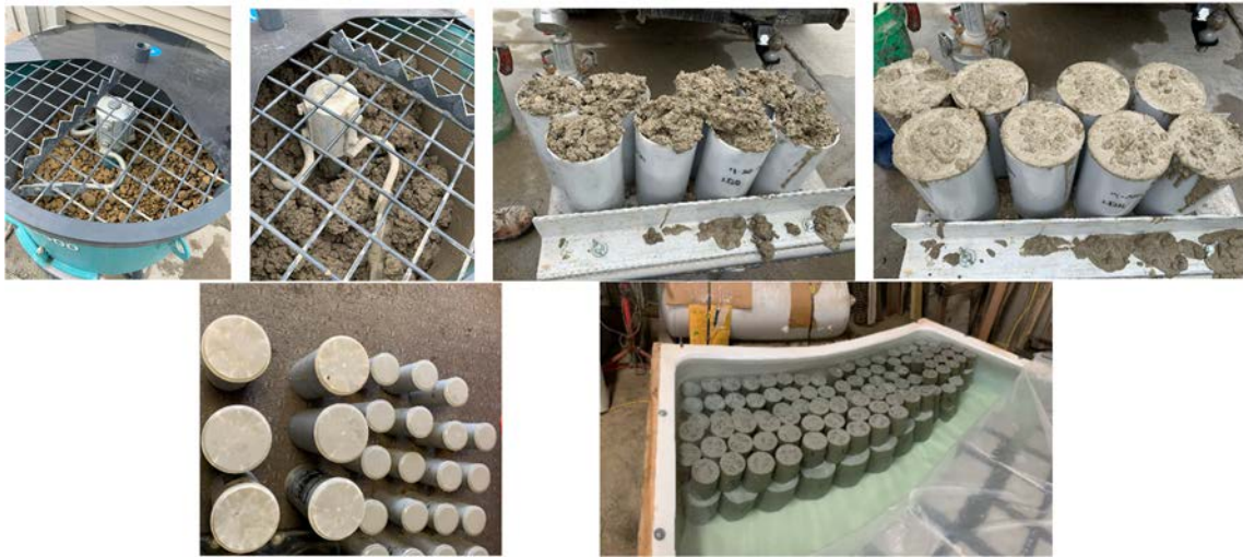
Figure 3.5: Picture of the various steps taken to prepare PCC test cylinders.
