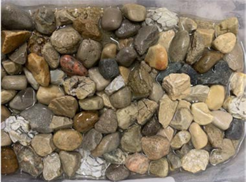
(e) Heterogenous composition of pit gravel leads to unpredictable out come
