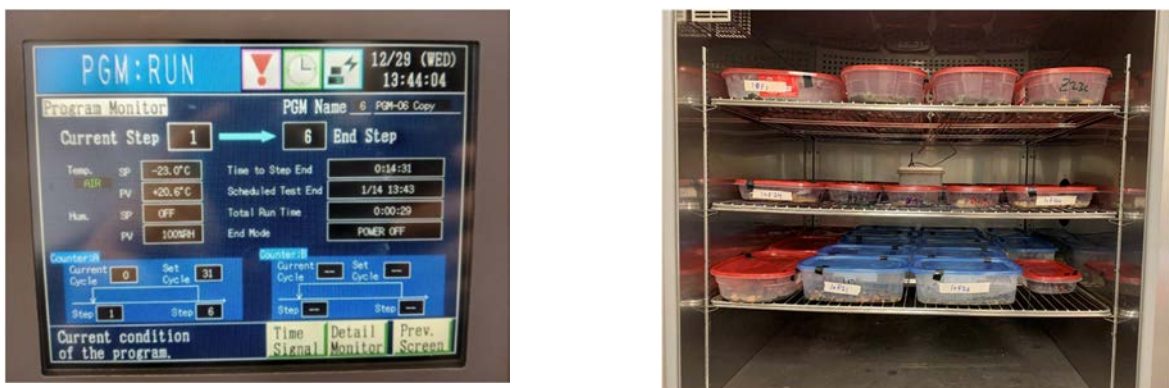
Figure 3.4: Freeze-thaw test systems used to process the investigated coarse aggregates.
