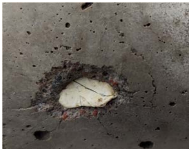
(c) Coarse aggregate initiate cracking in PCC cylinder surface
