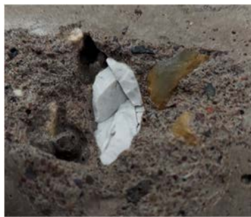
(a) Coarse aggregate fracture
