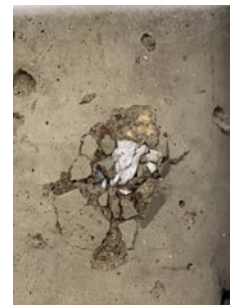
(c) Coarse aggregate initiate cracking in PCC cylinder surface
