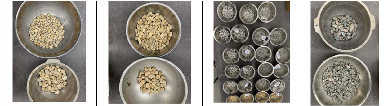
Figure 3.1: Pictures of typical calcareous (CLS) and dolomitic limestone (DLS) coarse aggregates used for this study.
