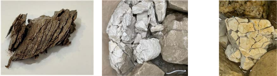
(a) Shale within DLS CA sample (b) Chalk within CLS CA sample (c) Chert within pit gravel CA sample
