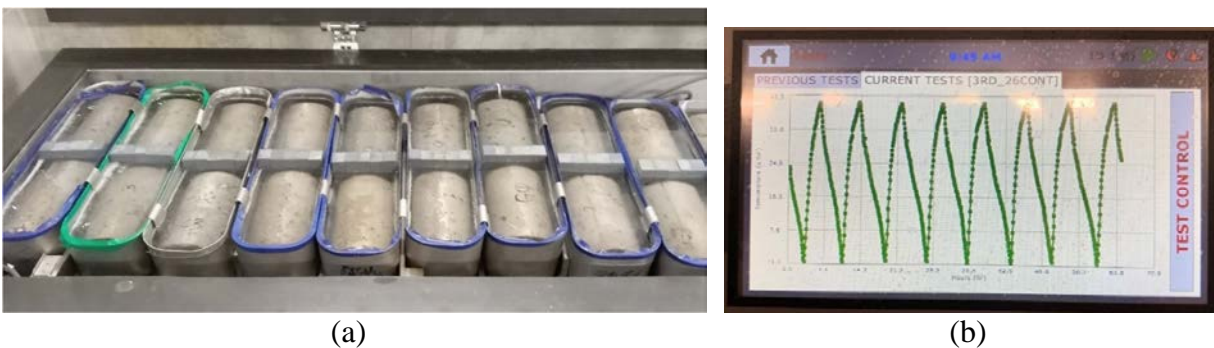
Figure 3.6: (a) PCC cylinders in frozen state inside the rapid freeze-thaw chamber; (b) The temperature-time freeze-thaw cycles applied to these cylinders.
