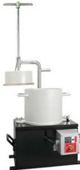
Figure 15. The VB apparatus used for experimental packing test
