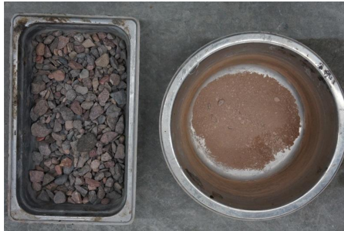
Figure 14. Fine material collected from coarse aggregate C2 by washing and drying
