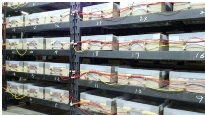
Rapid chloride exposure testing in progress.
