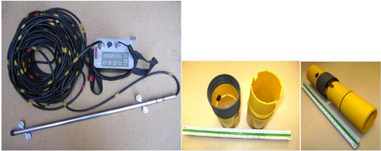
Figure 18. Typical slope inclinometer parts and inclinometer casing
