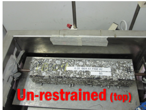
Figure 35. Picture of the Instrumented Asphalt Mixture Beam Prior to Mixture T_g Testing.
