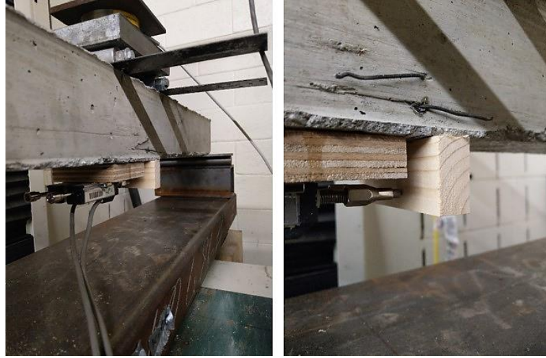
Figure 25 - Linear potentiometer set-up using woodblocks.
