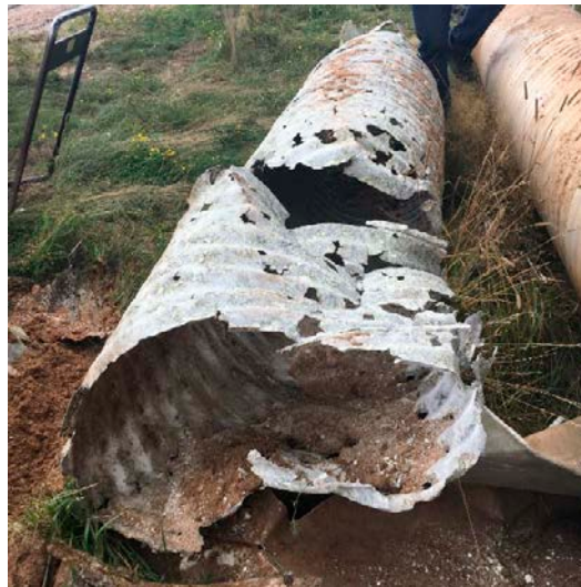
Corroded aluminum pipe removed from WIS 32
