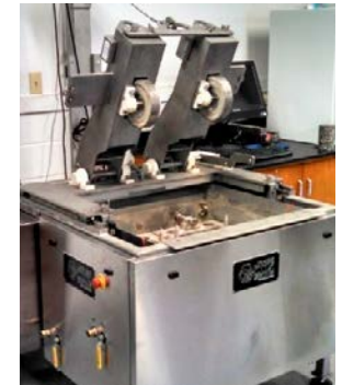
Specimen testing with (from left to right) DCT, IDEAL-CT and HWTT.
