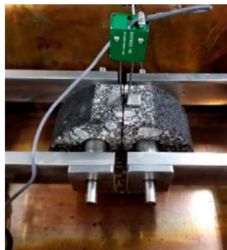
Specimen testing with (from left to right) DCT, IDEAL-CT and HWTT.
