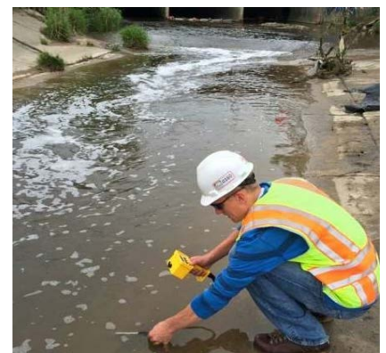
Handheld turbidity monitor used to collect data at runoff site.
