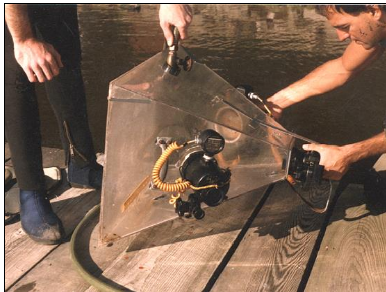
Figure 1.3.8.5-1: Inspectors Attaching a Clear Water Box to an Underwater Camera.
