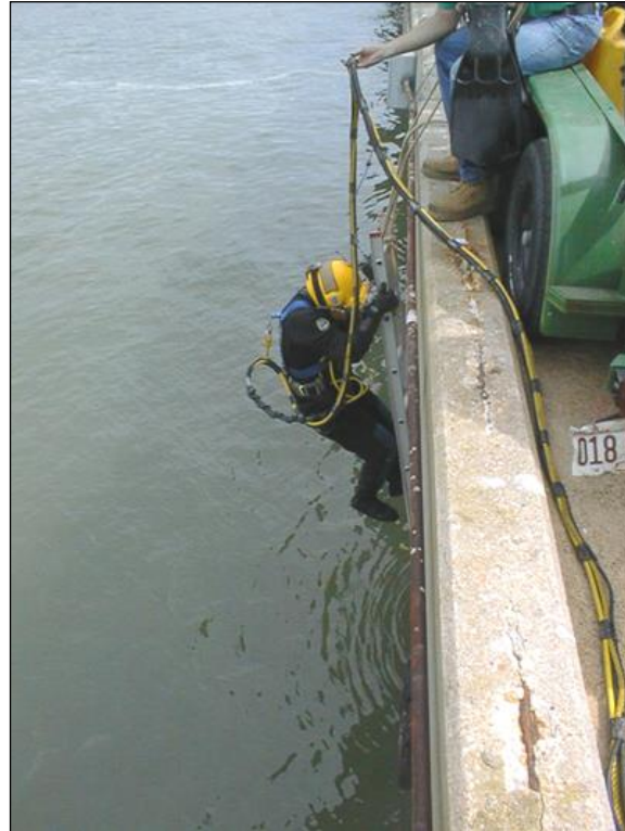
Figure 1.3.8.4-1: Inspector Using Surface-Supplied Air Equipment.
