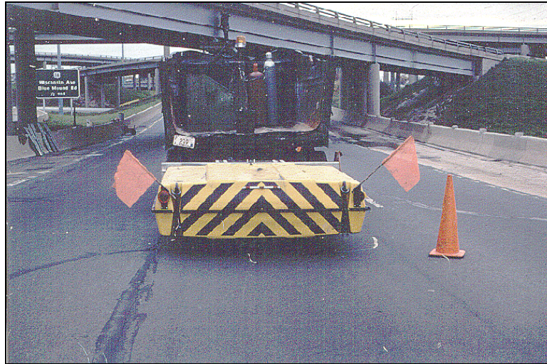
Figure 1.4.8.3-1: Truck Mounted Crash Attenuator.
