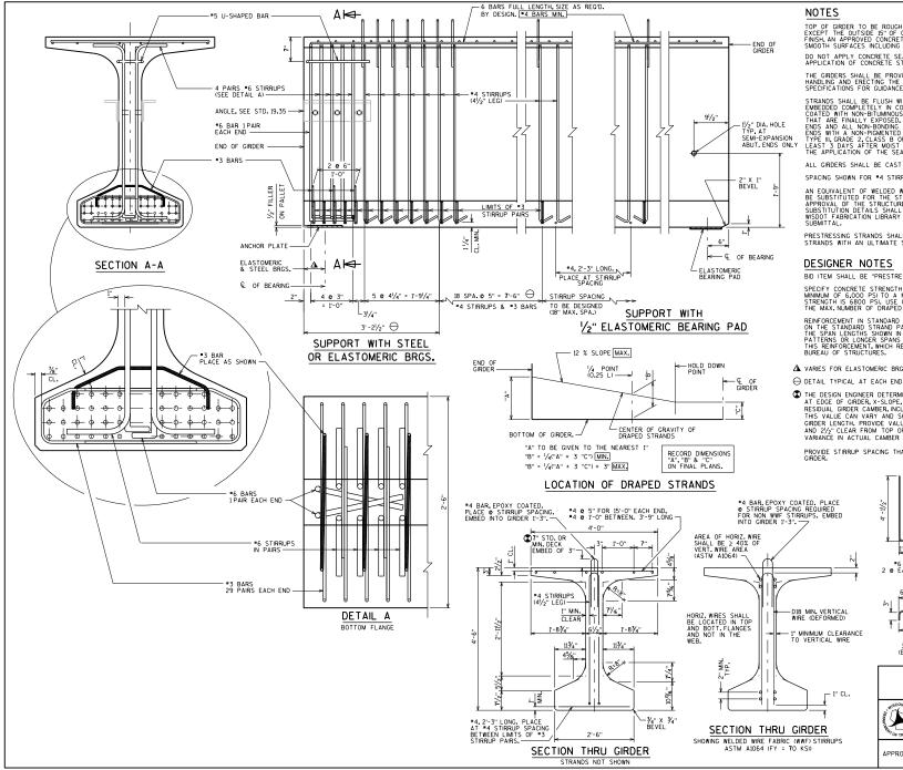
TOP OF GIRDER TO BE ROUGH FLOATED AND BROOMED TRANSVERSELY. EXCEPT THE OUTSIDE 15" OF GIRDER, WHICH SHALL RECEIVE A SMOOTH FINISH. AN APPROVED CONCRETE SEALER SHALL BE APPLIED TO ALL SMOOTH SURFACES INCLUDING THE OUTSIDE 15" OF THE TOP FLANGE.
