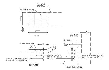
CONCRETE BEARING BLOCK DETAILS
