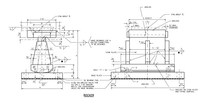
★ 400 K < REACTION < 1000 K. USE %" WELD. 1000 K < REACTION < 1500 K. USE ¾" WELD. \* FOR REACTION > 1000 KIPS USE 2" STIFFENERS.
