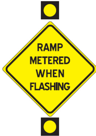
Figure 3.3.1 “Ramp Metered When Flashing” Sign
