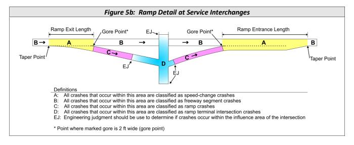
The definitions shown in *Figure 5b* for speed-change areas and freeway segments are based on definitions in the Enhanced Interchange Safety Analysis Tool (ISETe): User Manual, published May 31<sup>st</sup>, 2012 through the National Cooperative Highway Research Program (NCHRP). *Figure 5b* also includes guidance about defining ramps and the influence area of intersections, which are definitions specific to WisDOT business practices.
