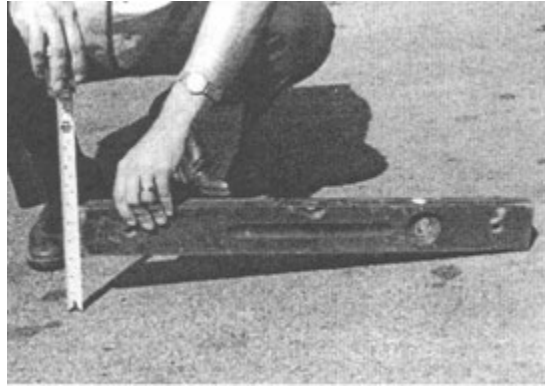
Figure 3. Measuring Super elevation with a Carpenter's Level (Source: Northwestern University Center for Public Safety)
