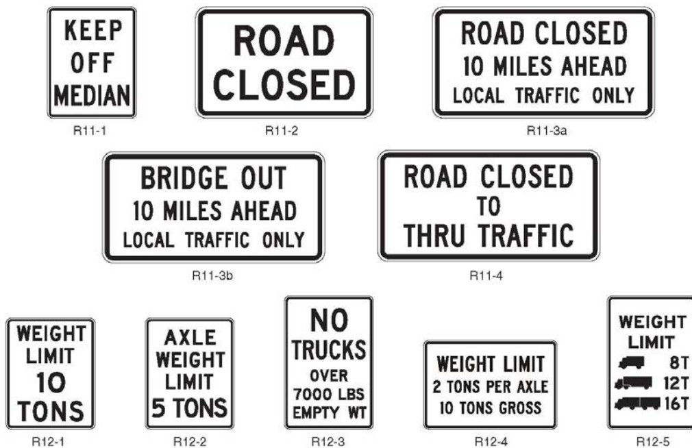
Figure 2B-29. Road Closed and Weight Limit Signs
