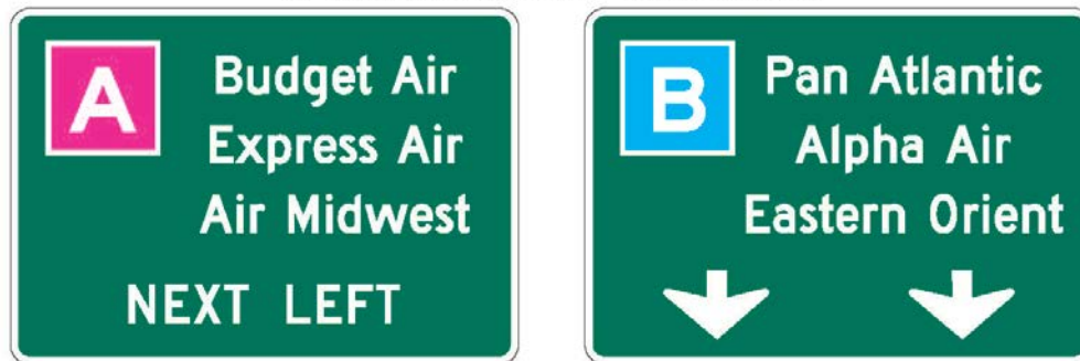
Figure 2D-1. Examples of Color-Coded Destination Guide Signs
