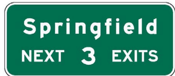
Figure 2E-33. NEXT EXITS Sign
