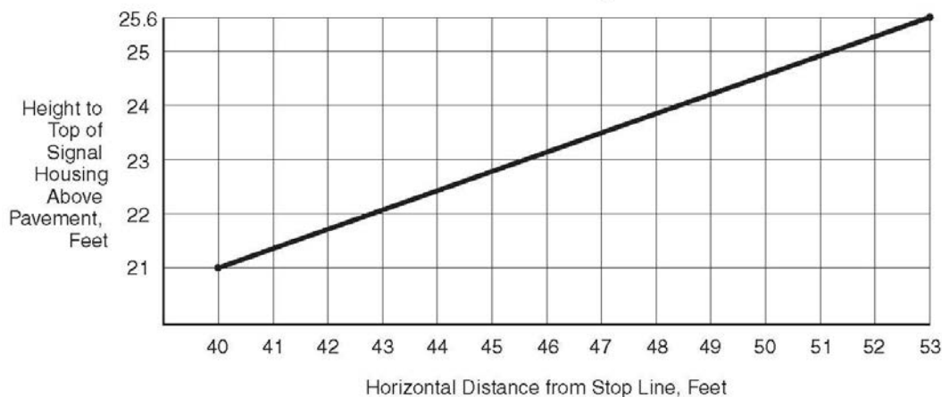
Figure 4D-5. Maximum Mounting Height of Signal Faces Located Between 40 Feet and 53 Feet from Stop Line
