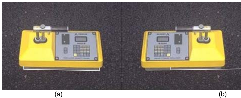
Figure 2: Nuclear gauge orientation for (a) 1 st one-minute reading and (b) 2 nd one-minute reading
