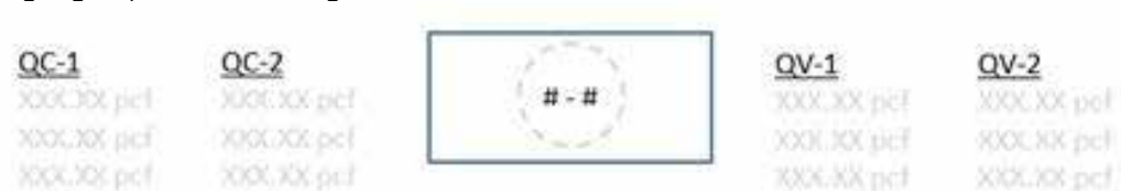
Figure 3: Layout of raw gauge readings as recorded on pavement
