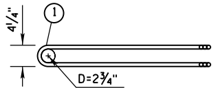
PLAN VIEW LOOP BAR ASSEMBLY (MARKED END SHOWN, INVERT FOR OTHER END)
