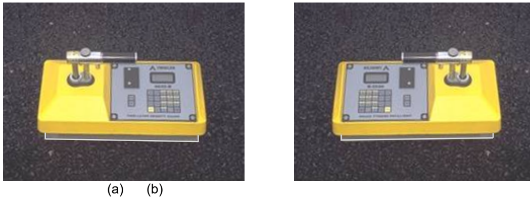
Figure 2: Nuclear gauge orientation for (a) 1 st one-minute reading and (b) 2 nd one-minute reading
